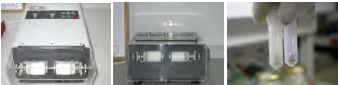
Figure 6. Two views of the electronic grinder (left) and two Eppendorff tubes with a seed and metallic ball (right) and the homogeneized endocarp fater grinding (left).
